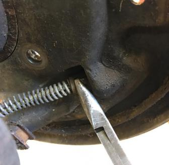
Disconnect the parking brake cable from the brake shoe, then remove and discard the brake shoes and hardware. The cable can then be removed from the backing plate by depressing its perimeter springs.
