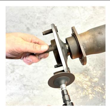
**Normally not required, but in rare cases** the OD of the axle shaft flange may be too large to fit inside of the supplied rotor. If this happens, the solution is to simply remove material from the outside of the axle flange with a sander while rotating the shaft as shown.
