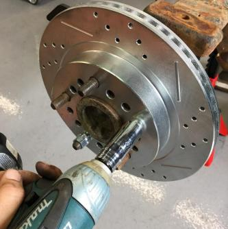
Bolt on the brackets using the supplied hardware as shown and torque to **20 ft-lbs**. Your caliper should be mounted to the **REAR** (back) of the axle. The rotor can now be installed using 2 lug nuts to temporarily secure it. In the case of drilled/slotted rotors, the direction of rotation shown is for the **passenger side**. **NOTE:** Verify that the rotors are sitting flat against the axle shaft.
